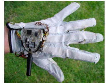
Ryan’s glove translates the finger movements of American Sign Language into written English.
